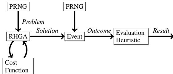
Figure 3: Simulation model. A pseudo-random number generator (PRNG) generates simulation scenarios in which the RHGA uses some cost function Cost 1 to determine a solution (where tugs should move). The PRNG then generates an event of drift, which depending on the current position of the tugs may be critical or not. The outcome (saving or not saving the drifting ship) is then quantified as Cost 2 by an evaluation heuristic.
